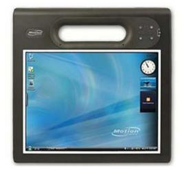
The Motion F5te is a rugged tablet which means it is more durable than a commercial tablet. Rated at IP54, it can take bumps, drops or exposure to wind, heat, and rain. The Motion F5 also has typical rugged
